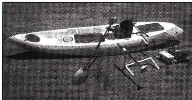
Cobra kayak together with fish tracking equipment (hydrophone, acoustic receiver and battery pack)
